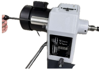
Figure 7-8: removing spur center
