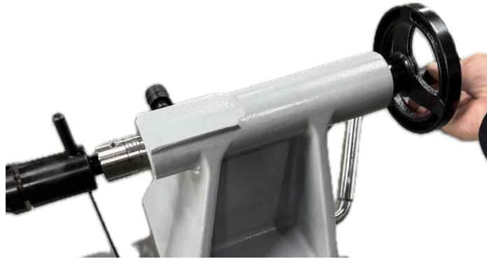
Figure 7-9: installing live center
