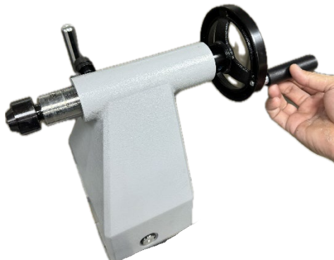
Figure 7-9: installing live center
