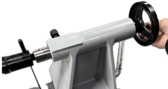
Figure 7-9: installing live center
